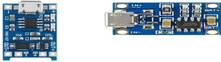
Fig. 10 Battery Charging Module
